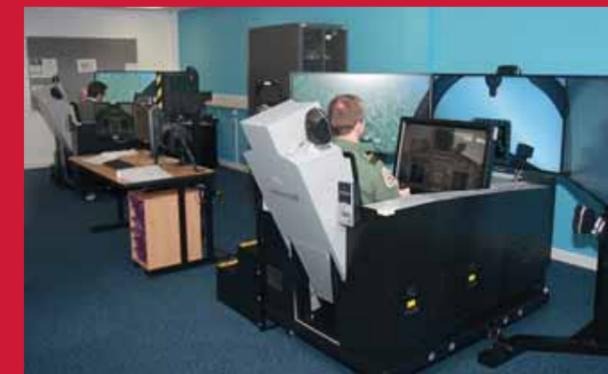
Flying training devices offer a step up in realism, constituting a fully-representative T2 cockpit for practising checks and procedures, and rehearsing missions covering the majority of UK airspace and airfields.
