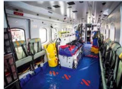
A customised stretcher stowage and plinth installation for casualties on the S-92 features a raised box on to which a stretcher is lifted to reduce the physical strain on rescue crews, and ensures the casualty is not too close to the floor. *Geraint Thomas via Bristow Group*
